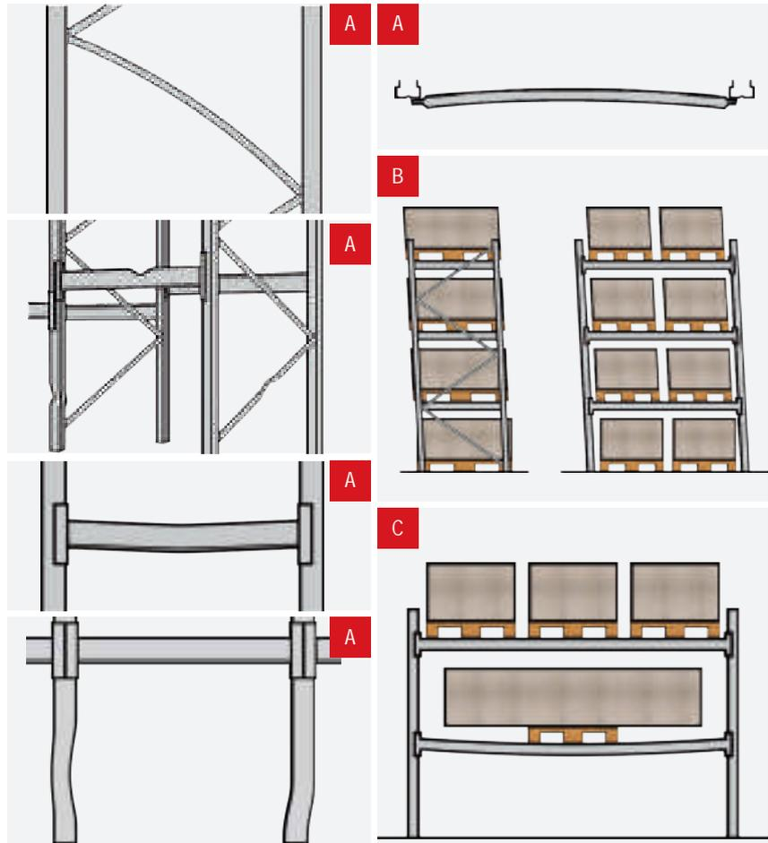
**A Deformation.** Even slightly bent beams and uprights can be a sign of potential danger. Beams and uprights with dents must always be replaced. **B Inclination.** Maximum inclination of an empty rack is 2,8 mm/m. For a fully loaded rack, it is 7,8 mm/m. **C Load weight and placement.** The weight of the load must not exceed max weight capacity, or be misplaced.
